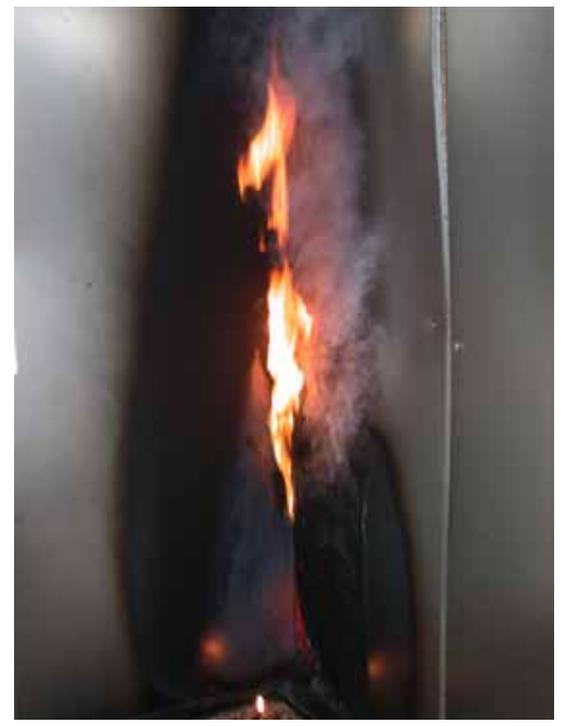
Ignition of pyrolysis gases at the opening
