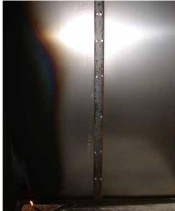
Flat bar in front of the joint between the two pieces of steel sheet (long wing)
