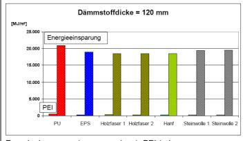
Energieeinsparung (energy savings), PEI (primary energy content), PU (Polyurethane), Holzfaser (wood fibre), Hanf (hemp), Steinwolle (stone wool)
