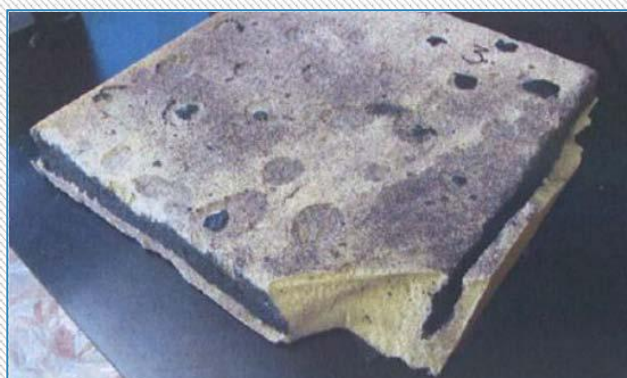
Picture 5: PU specimen removed from the flat roof
