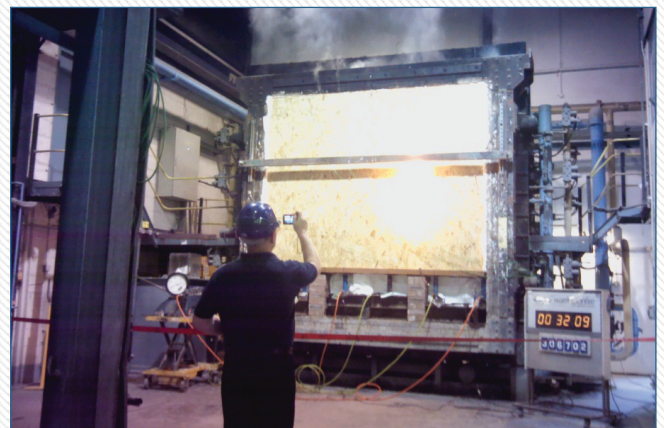
Figure 3: Mineral fibre test 306702 failing at 32 minutes
