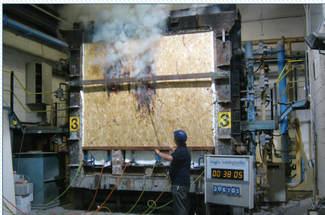
Figure 2: PIR test 306703 failing at 38 minutes
