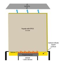
Experimental test method: equipment and test conditions
