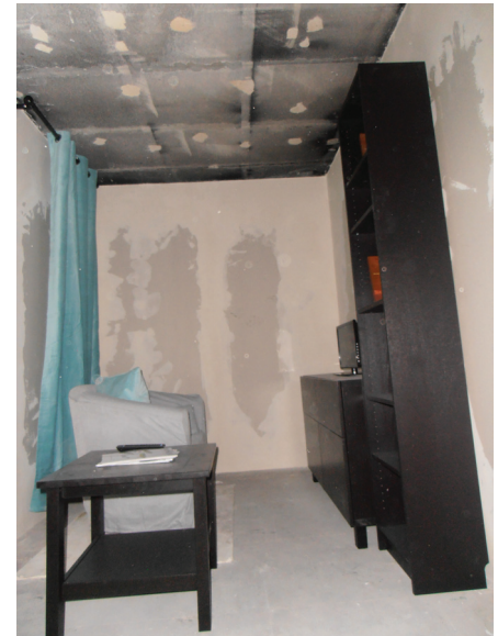
Test room according to ISO 9705, also referred to as Room Corner Test
