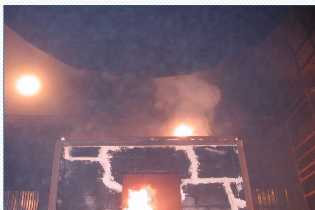
Figure 3: Substantial smoke release through the roof
