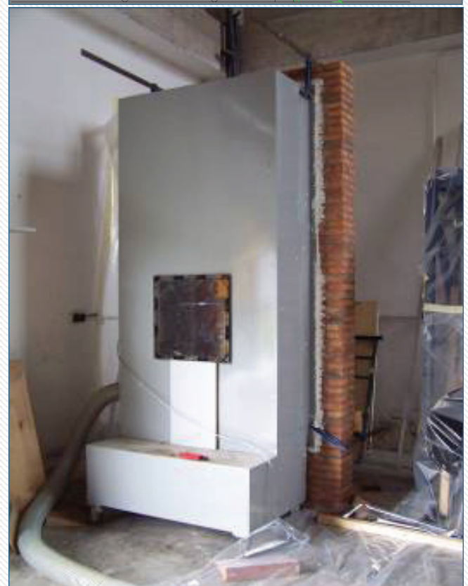
Figure 2: pressure chamber attached to test specimen
