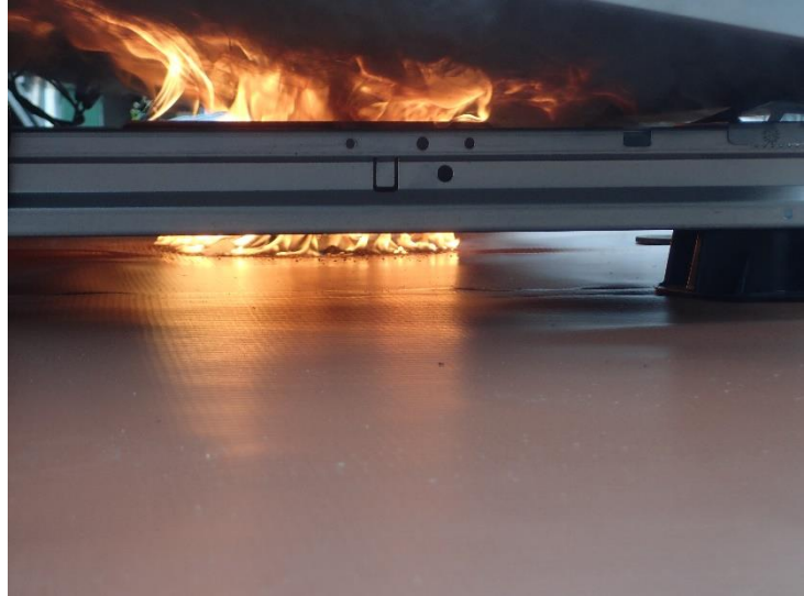
Photo 7 The roofing and PV module are burning (time 10:11).
