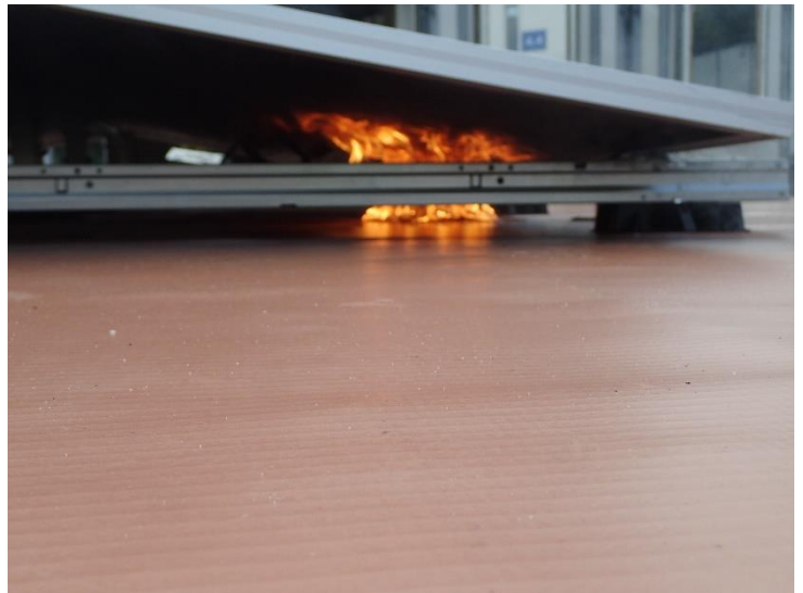
Photo 27 The roofing and PV module are burning (time 15:04).
