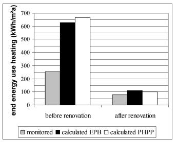
Figure 3 Comparison of end energy consumption for heating
