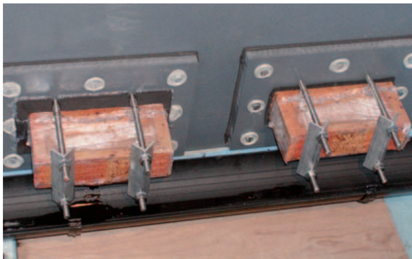
Figure 6.1 Pressed facing bricks being tested
