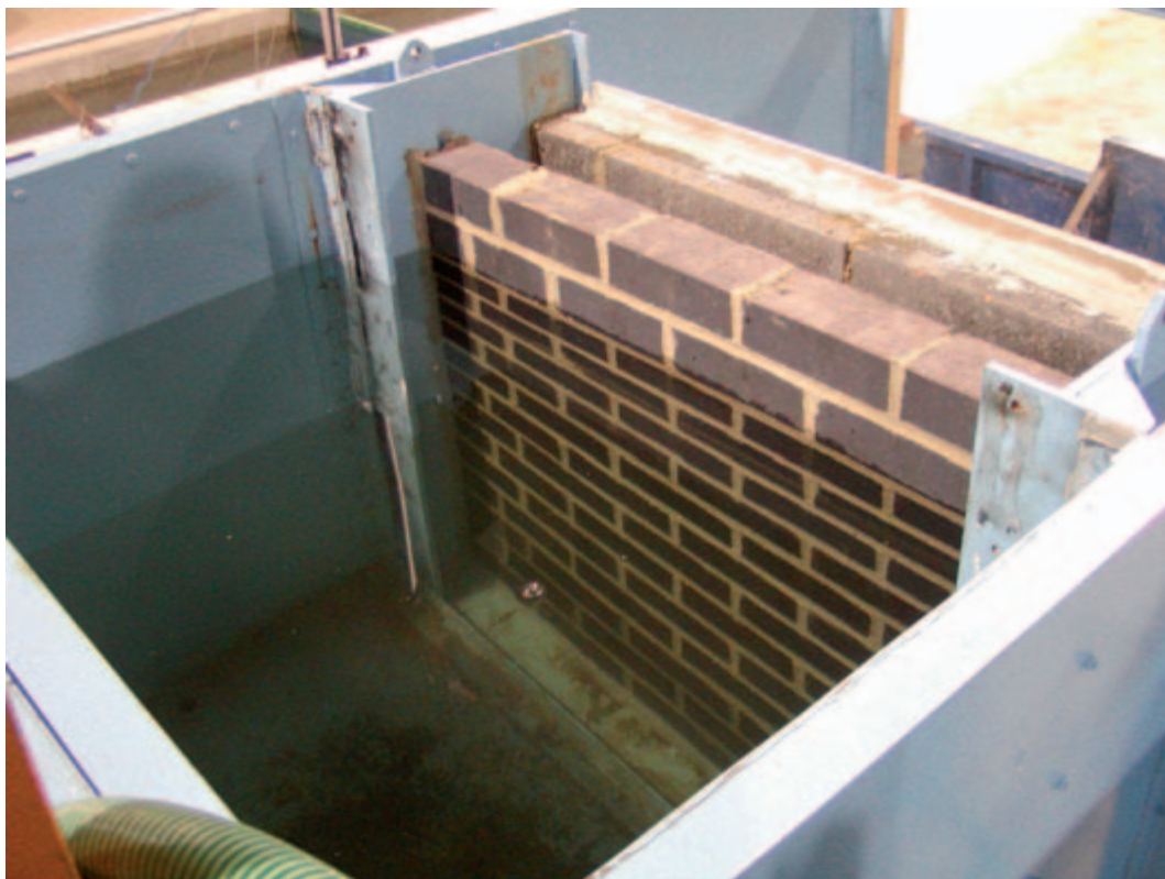
Figure 7.5 Testing a cavity masonry wall
